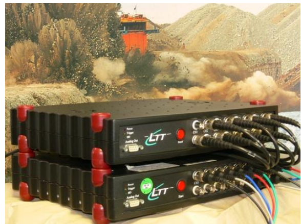
Figure 3: The rugged transient recorder series LTT-184 and LTT-186 have delivered high performance under harsh conditions including detonation tests on shore and on sea.
