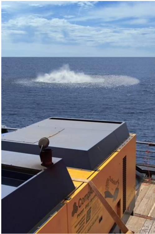
Figure 2: Test detonation with lower explosive charge. In the foreground the CompAir compressor that generates compressed air to produce the bubble curtain [2].
